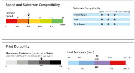
Videojet evaluation of observed performances of the Rough Texture Ribbon with optimized printer setting and receptors.
